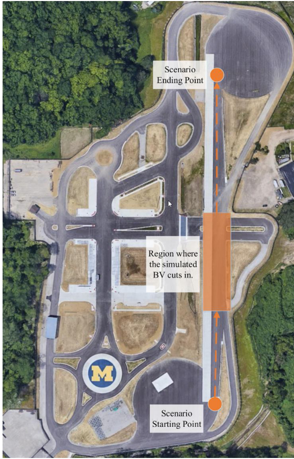
Fig. 6. Bird's-eye view of the cut-in test scenario at Mcity.
